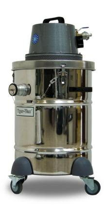
Stainless steel SAE 430 body and recovery tank. Contains a true HEPA Filter (H14) located upstream. This unit is static dissipating and conductive (Category 3 - Zone 22 (Dust)) and can be used for general maintenance. This unit cannot be used to recover conductive or combustible dusts or flammable liquids. With a powerful suction this unit is designed for industrial applications. All of our HEPA vacuum cleaners are Aerosol Leak Tested before leaving our facility.
