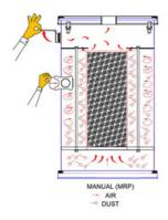
The Manual Reverse Purge (MRP) System allows the operator to not have to open the vacuum cleaner in order to clean the Cartridge. By opening the Reverse Purge Atmospheric Pressure Release Valve the Cartridge is automatically purged of dusts. This Purging System reduces maintenance down time.
