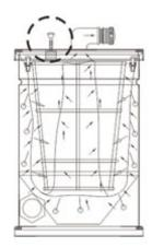
The Manual Fitler Shaker system allows the operator to clean the main filter without having to open the vacuum cleaner. This shaker System reduces maintenance down time.
