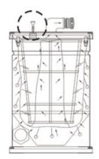
The Manual Fitler Shaker system allows the operator to clean the main filter without having to open the vacuum cleaner. This shaker System reduces maintenance down time.
