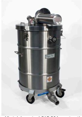
All stainless steel SAE 304 construction. Less than 10 Ohms of resistivity. This unit is equipped with a true HEPA Filter (H14) located downstream. This is a wet & dry vacuum cleaner. Recovery tank capacity of 40 gallons (152 liters) - dry and 45 gallons (171 liters) - liquid. All of our HEPA vacuum cleaners are Aerosol Leak Tested before leaving our facility.
